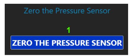
If a pressure sensor is present in the ADCP, the pressure sensor should be zeroed before being deployed. This button will zero the pressure sensor.
