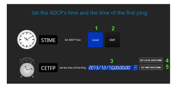
This section will allow the user to set the ADCP time and the time of the first ping. The ADCP time can be set to Local or GMT. The Time of First Ping is the when the ADCP should begin collecting data. This date and time can be set to the future so batteries will not be wasted while transporting it to the location for deployment.
