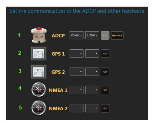
If the user selected the SeaTrak ADCP type, then additional fields will be available here to allow the user to record additional navigational instrument data to the project.
