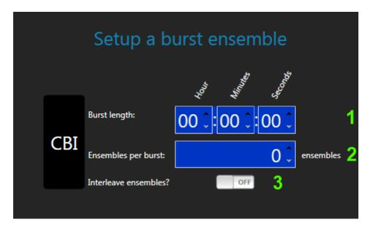
Burst mode pinging allows the timing to change from the standard way of pinging. With burst mode pinging, each subsystem configuration is given an time length to ping and wait until the next subsystem configuration begins pinging. This can be useful when strict timing for the data collection is required. With the standard mode, the pinging would occur at a fixed rate. In burst mode pinging, the data can be collect in time blocks with gaps in blocks included.
