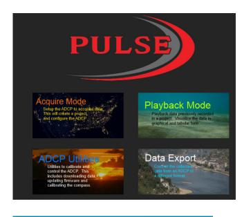
When the Pulse application is started, the application will start on the Home page. The Home page allows the user to connect to an instrument or select a Project to playback.
