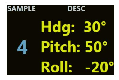
In this example, this is the 4<sup>th</sup> sample point. It is telling the user to have Beam 0 of the ADCP point to 30 degrees. Give a pitch of 50 degrees and a roll of -20 degrees. Once the ADCP is in this position, press the "Next Sample" button. When the compass reads this position, it will then move to the next sample.
