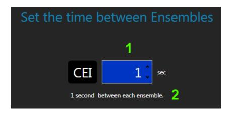
The Time Between Ensembles is how often data will be output from the ADCP. The ADCP is configured to collect data. The data will be output to the computer or recorded to the internal storage based a rate based off this value. This value is also sometimes referred to as the *Ensemble Interval*.
