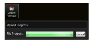
Upload the latest firmware to the ADCP. This will allow the user to upload any files including firmware to the ADCP's internal memory. Press the "Update Firmware" button and select the file you would like to upload. Then press OK. Wait for the file to be uploaded to the ADCP.
