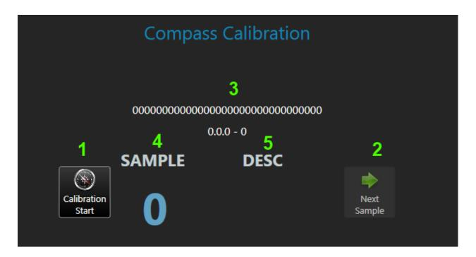
The compass calibration is required in the field to ensure the compass will not be affected by its environment. The calibration will take 12 samples. The application will then prompt when the calibration process is complete.
