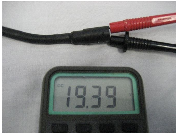
Figure 9: Test Power on Underwater Connector
