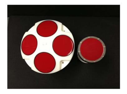
As another example, the image following shows a 300KHz Janus head ADCP (left) and a 150 KHz Doppler Array (right). Note that although the Doppler Array is approximately half the frequency, it is roughly the same size, weight and volume as the 300 KHz system, but the 150 KHz system has twice the profiling range.
