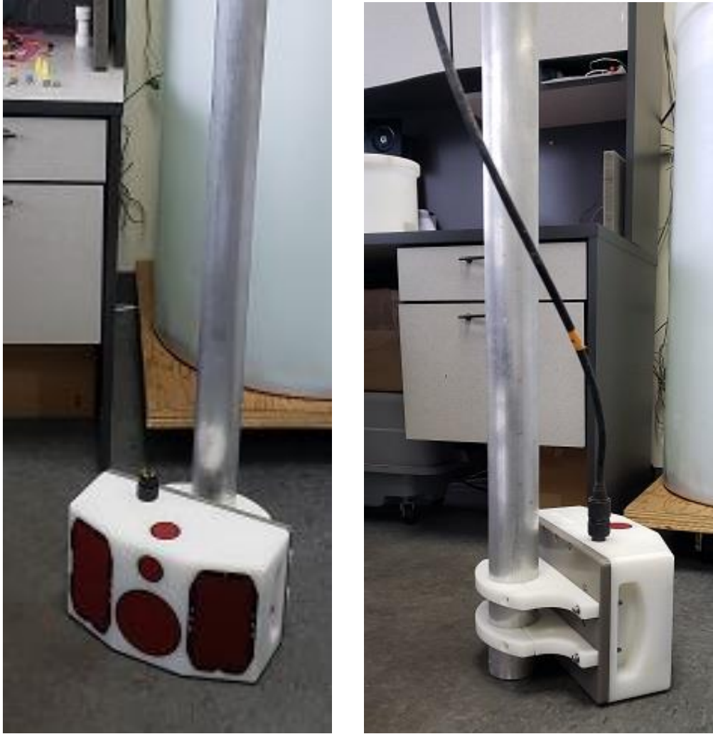
Figure 28. HASCP mounted on a pole used for internal testing at RTI.
