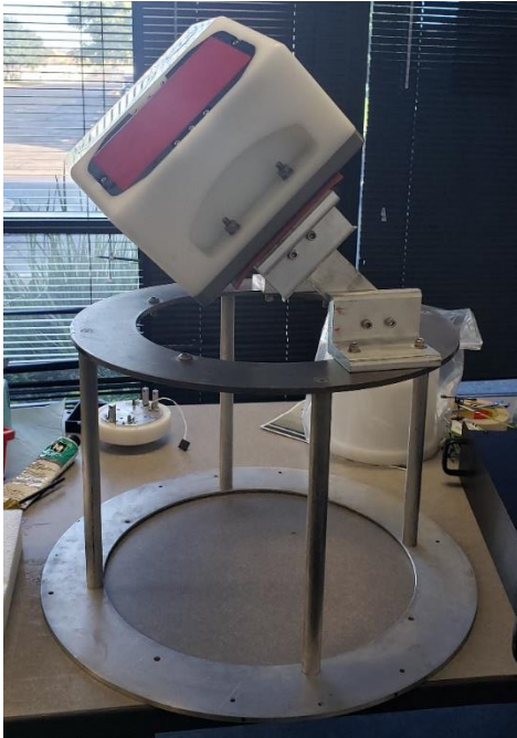
Figure 18. Fixture used for mounting the HASCP at the lake. The instrument was mounted at an angle of 45 degrees with all the beams facing down at the lake.
