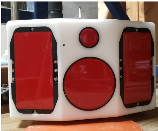
Figure 17. Front view of the HASCP showing the two-1200 kHz rectangular transducers, a single-4 inch 600 kHz piston transducer and a single - 2.4 MHz piston transducer.
